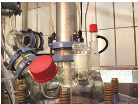
Figure 6. Gas flow measurements on large and small scale. For the 10 L reactor (left) the constriction device was a 60 mm glass pipe, i.d. = 3.0 mm, mounted at the small red GL cap in the reactor lid. The black silicon tubing to the differential pressure probe is visible below the pipe. For the 4 mL GC vial (right) the pressure difference was measured over a 60 cm coiled PEEK tubing (inner diameter 0.25 mm).
